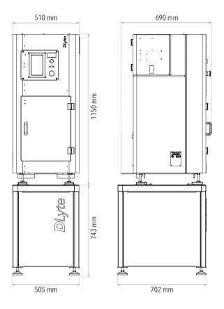
Anti vibratory support included. Also includes the dental holder head designed to hold holder finger, bars, crowns, attachment, spring and wire.
